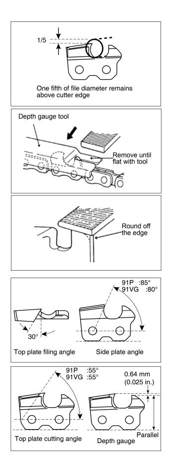
Place the depth gauge tool firmly on guide bar so that depth gauge protrudes. Then file top of depth gauge with the flat file until flat with top of the depth gauge tool.
